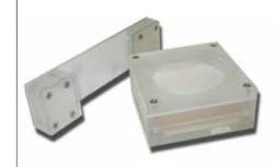
The QUART dentil test phantom is designed to be used for QA/QC routine testing in conventional Dental X-Ray applications ranging from intra-oral to panoramic and cephalometric equipment. It was developed to fully test equipment featuring film-screen technology.
